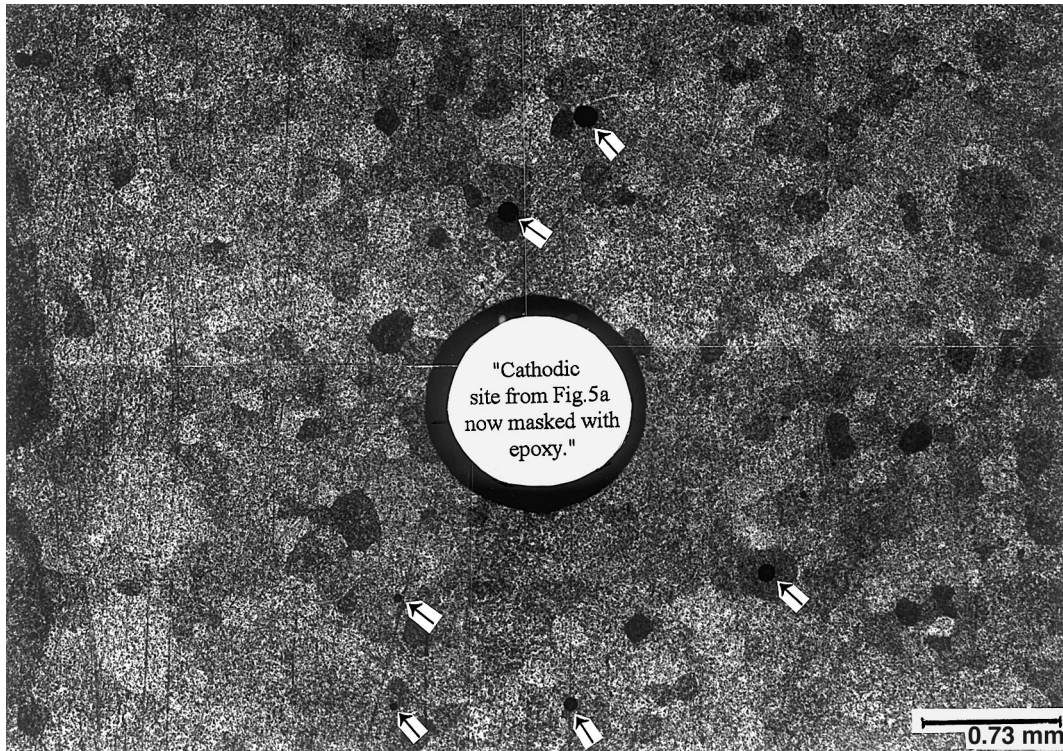
Fig. 6. Minor sites active after major site (shown in Fig. 5) was masked. Arrows indicate Cu deposits (optical micrograph).
